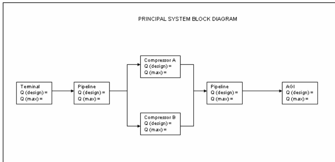
An expanded version of this could be used to identify where spare capacity exists by representing all of the primary assets on one complex diagram. This could show a comparison of the design capacity of each asset with the maximum expected throughput (for example under the Base Case supply, 1 in 20 peak day demand conditions).
