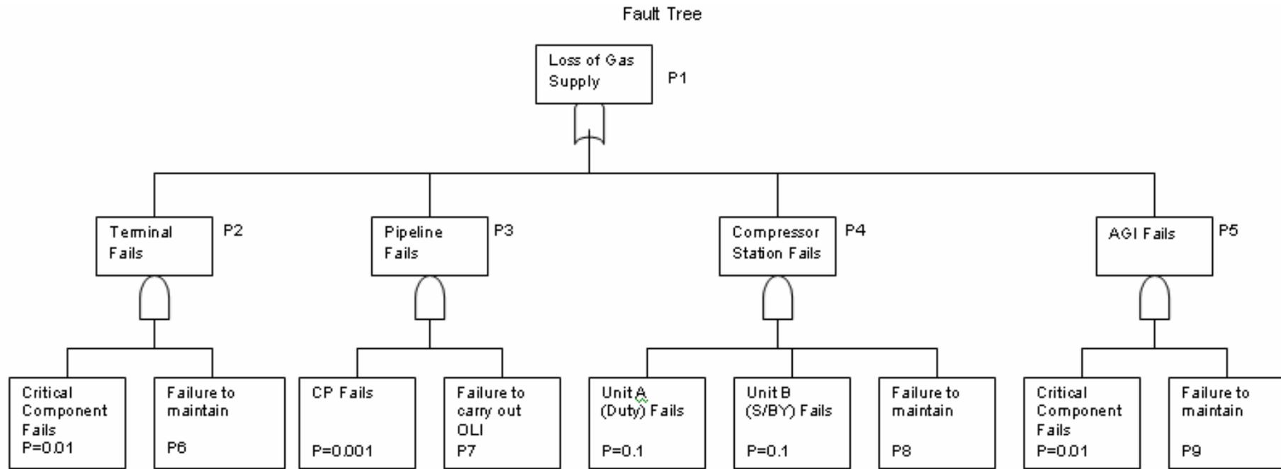
The principal assets appear in the order shown a number of times in the NGG network and hence many of these could be produced for discrete sections of the network. The top event, namely loss of gas supply occurs if any of the principal assets fail. The probability of this loss occurring will be significantly dependant upon maintenance and equipment sparing (or redundancy).
