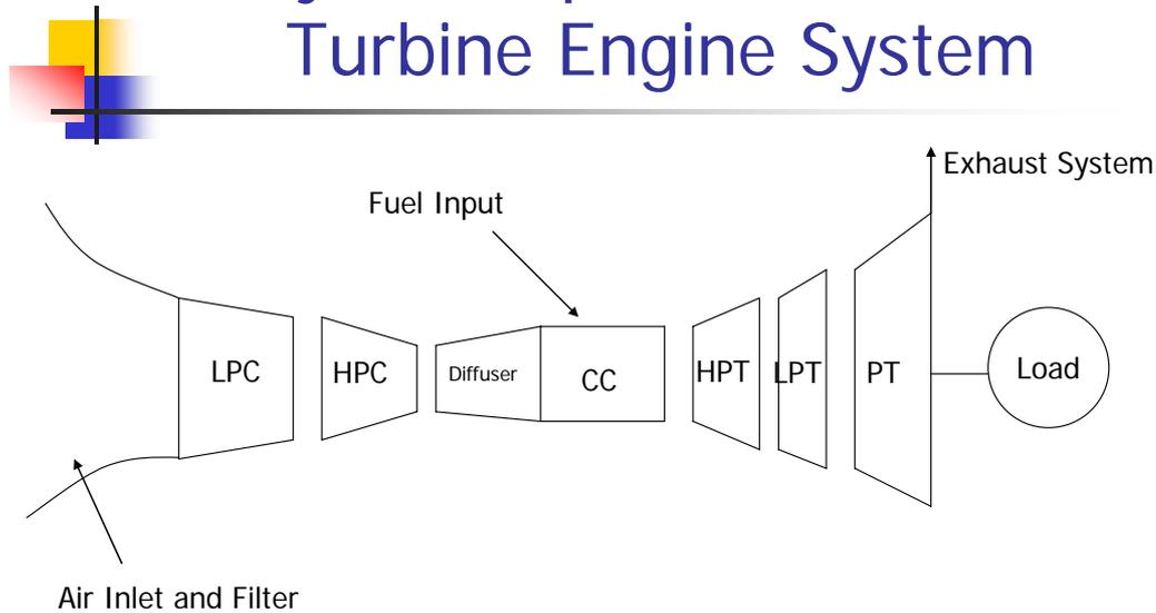
Fig 3: Typical Layout of a 3 Shaft Gas Turbine System
